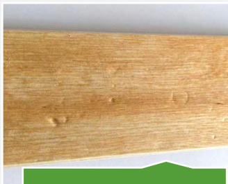
pressure marks in 5 mm diameter
