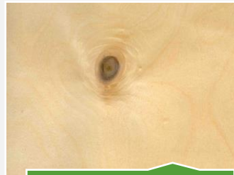
dark knots 10 mm, repaired if needed
