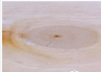
light sound knot in diameter max 25 mm
