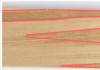
different contrasting colour shades on one slat up to 10%
